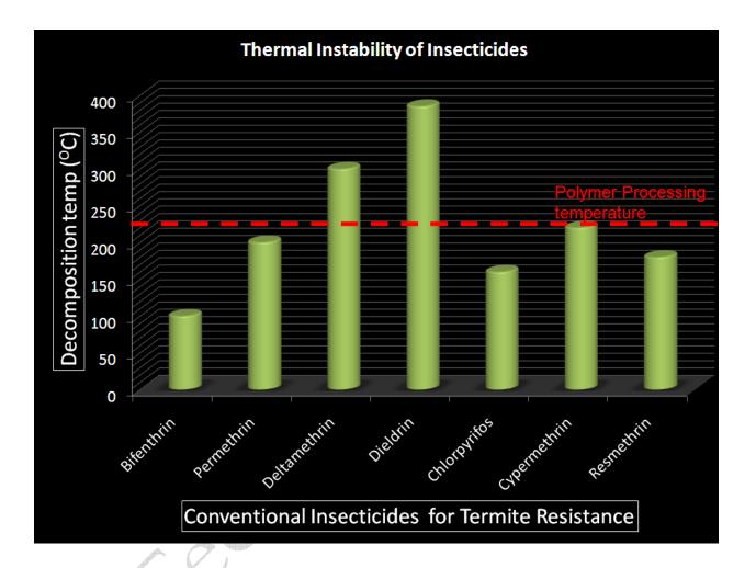
The thermal degradation temperature of Deltamethrin is 320°C which is in the same range as the process of extrusion. Elevated as well as localized temperatures in an extruder can go as high as 400°C and even beyond. This can result in serious problems for workers which will be handling the product. Moreover the temperatures are quite high near the tube exits of the
