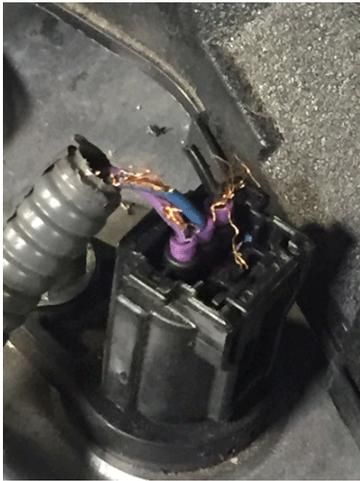
Many new vehicles now use wiring that has a soy-based coating, which is better for the environment and cheaper to make than the traditional kind.
